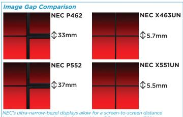
NEC's ultra-narrow-bezel displays allow for a screen-to-screen distance between two neighboring displays as thin as 5.5mm, close to 450% improvement compared to its previously revolutionary P Series displays.
